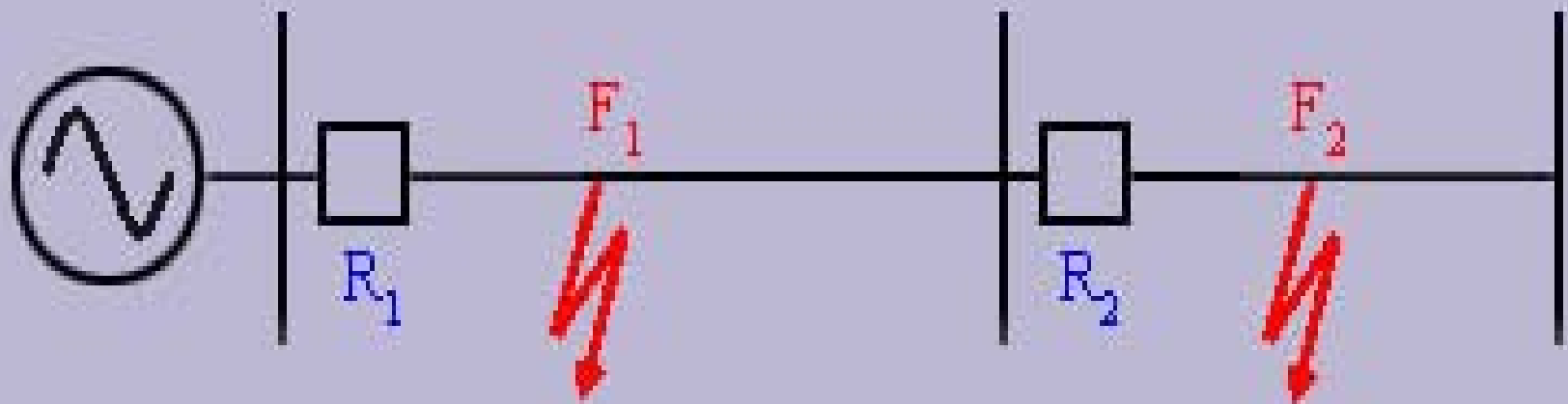
Fig 2.1 Radial Distribution System
